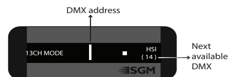
Figure 8: Set DMX address
