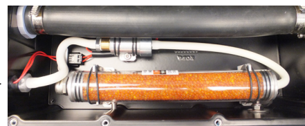
Silica gel desiccant in tube in the fixture head
