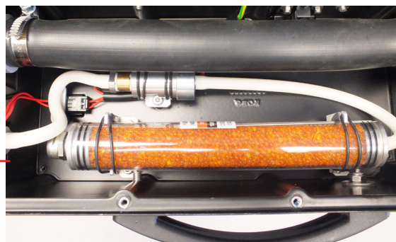
Silica gel desiccant in the fixture base
