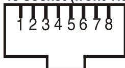
RJ-45 socket (front view):
