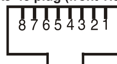
RJ-45 plug (front view):
